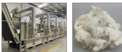
Fig. 1: The textile shredding machine (left) and defibred cotton (right)
